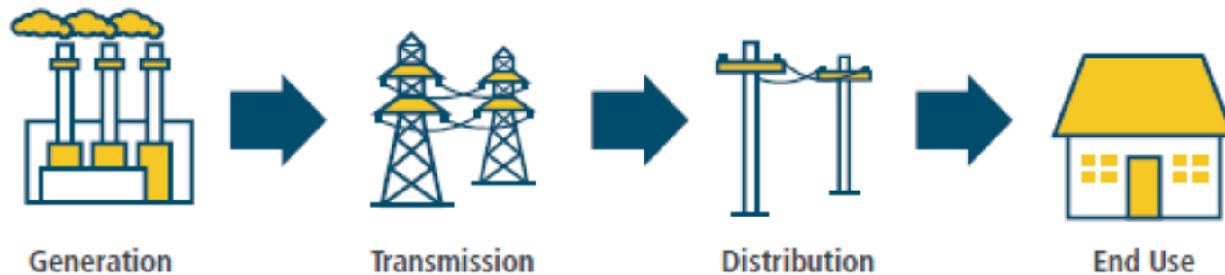
Figure 1-10. Traditional One-Way Flow Electricity Supply Chain 75
